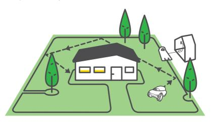
The mower moves randomly within its working area, as defined by the perimeter wire. This kind of random movement provides the perfect cut and ensures complete coverage of your lawn. In addition, it centers itself on top of the perimeter wire to ensure accurate, flawless edging.
