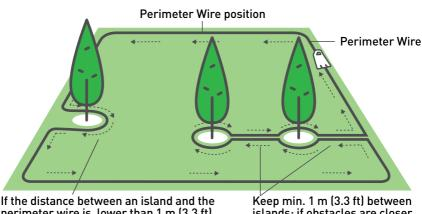
If the distance between an island and the perimeter wire is lower than 1 m (3.3 ft), make the obstacle part of lawn's edge.
