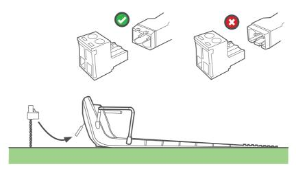
Insert only two stakes into the Base Station holes as shown.
