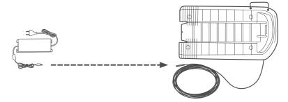
Make sure the connector is inserted the whole way up to the white mark.
