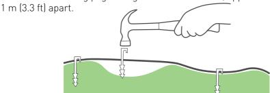
Hammer the extension cable into the ground so it's not a tripping hazard.
