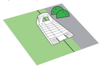
In case of External Installation, the Base Station should be placed in a small shift to the right, in order to allow smooth entry of the mower to the Base Station.
