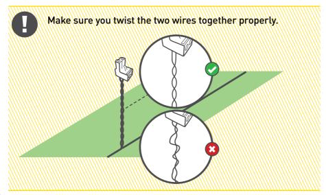
Strip back 5 mm (0.2 in) of insulation from the wire ends, insert the twisted wire into the connector and secure it using a small flat screwdriver.
