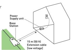
Connect the DC cable from the Power Supply unit to the 15 m (50 ft) extension cable.
